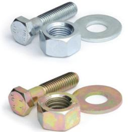
**Hot-dipped galvanized steel** has a thicker zinc coating for better corrosion resistance, making it suitable for outdoor use. Because of the thick plating, only galvanized nuts and washers will fit galvanized bolts. The coating typically has a rough, dull grey finish.
