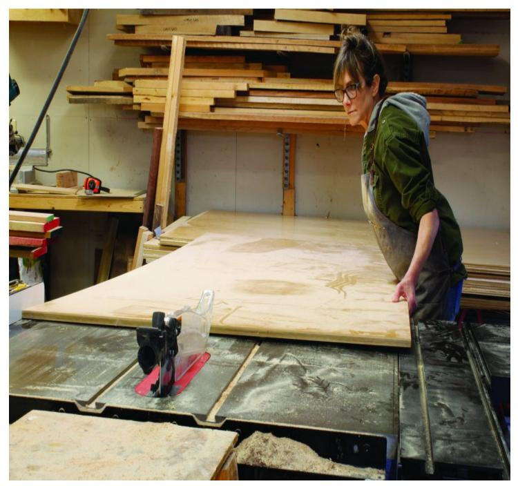
Rip first. I store my plywood on sturdy sawhorses near the table saw so that I can pull one end of a sheet over to the edge of the saw, adjust it against the fence and rip.
