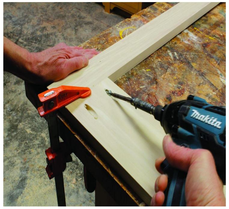
Pocket the difference. A pocket screw jig makes strong face-frame joints quickly. You can buy a special clamp to hold the rails and stiles in place, but I simply clamp the parts together on my bench, making sure they're square.
