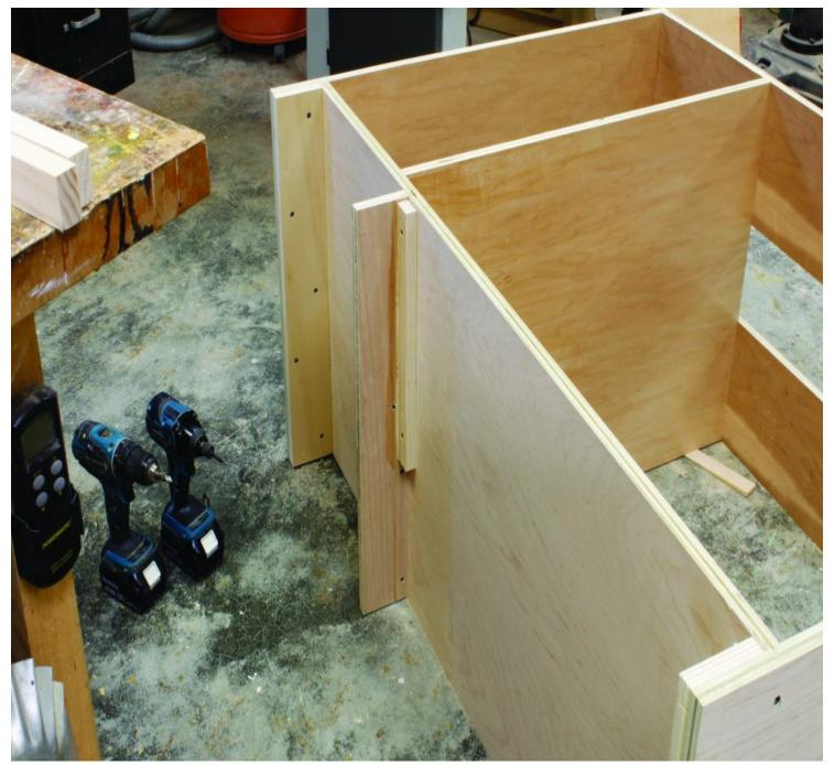
Intermediate support. A batten screwed to each side of the foot allows you to attach it to the cabinet's underside. I stagger the battens, putting one toward the front, the other toward the back, so that I can screw into them from the opposite side of the support foot.
