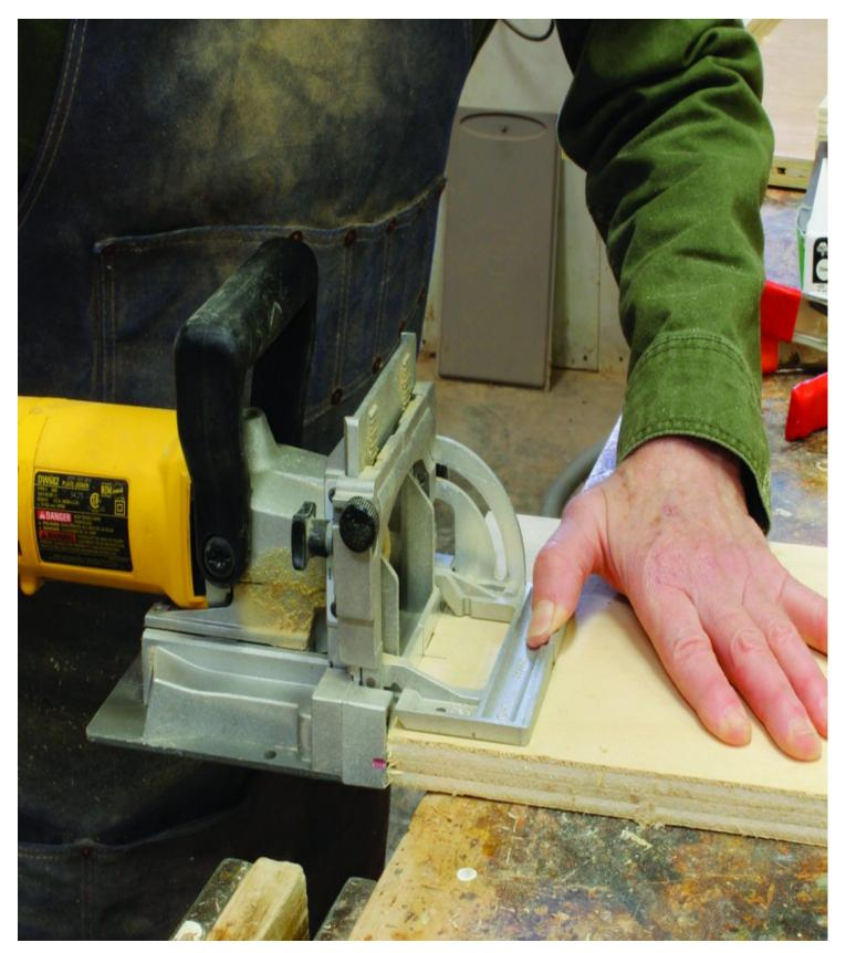
Flat and firm. Clamp the top (whether it's solid or strips) to your bench and hold the biscuit joiner firmly in place, then make the cut.
