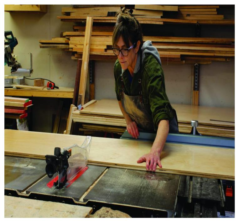
Be there and be square. A sliding table set at 90° makes it easy to cut the first end of each casework part square. You can then cut multiple parts to the same length by crosscutting with the rip fence.
