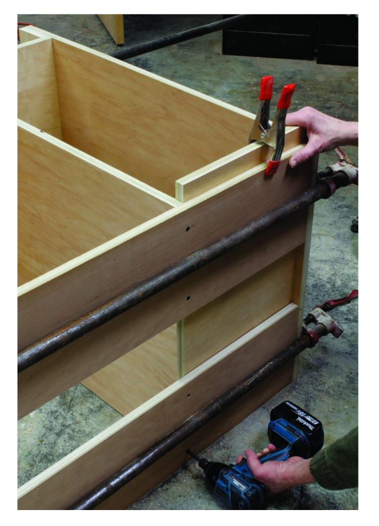
Spacers for the win. Use a piece of scrap plywood to lay out holes for vertical dividers and locate them for fastening. Then rely on the scrap to locate the divider while you drill pilot holes with a countersink/drill bit and screw it in place.
