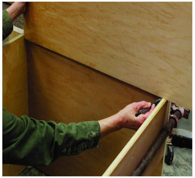
Direct measure. Determine the length of dividers by holding one end against the cabinet floor, then marking the other. Because it's typical for floors and tops of wide cabinets to sag or bow, measure for dividers at the nearest end. That way your divider will even up the height of the cabinet near the center.
