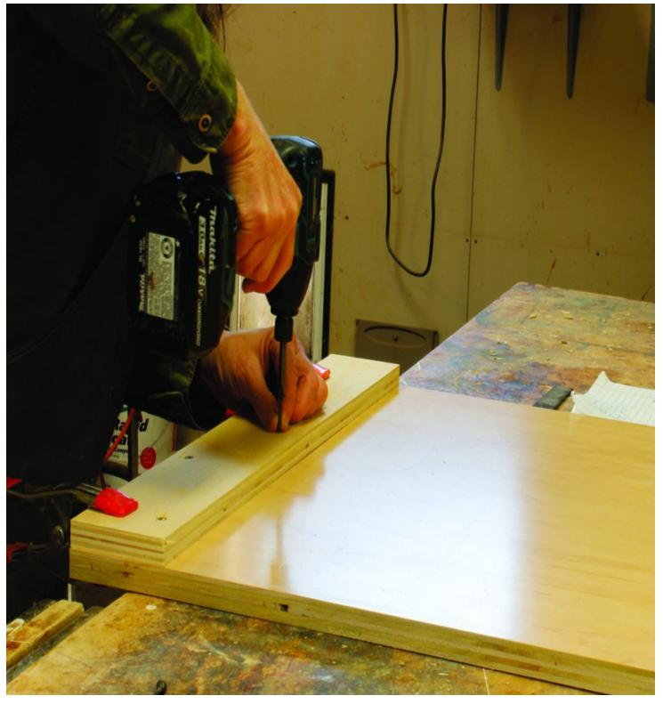
Simple and strong. Clamp the spacer in place at the bottom of the cabinet side and attach with 11/4" Twinthread screws. Four or five are plenty for each side of a typical base cabinet. You can predrill and countersink or use an impact driver, as I did here.
