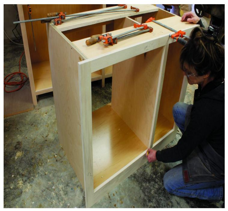
Direct measure again. For vertical dividers, wait until you have the main part of the face frame screwed together. Clamp (without glue) to the carcase. Hold one squared end of the divider stile in place and mark the other, then cut.
