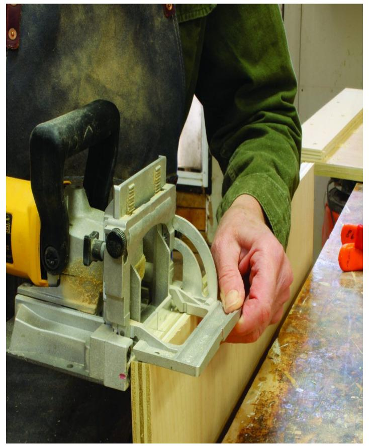
Steady on. For safety and accuracy, clamp the cabinet side in your vise and hold the biscuit jointer firmly against the fence to make a square cut.
