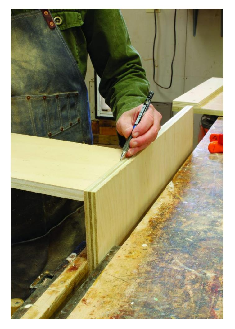
Top joint. In most cases you can simply hold the strip in place and mark the center line for each biscuit from the strip to the cabinet side.
