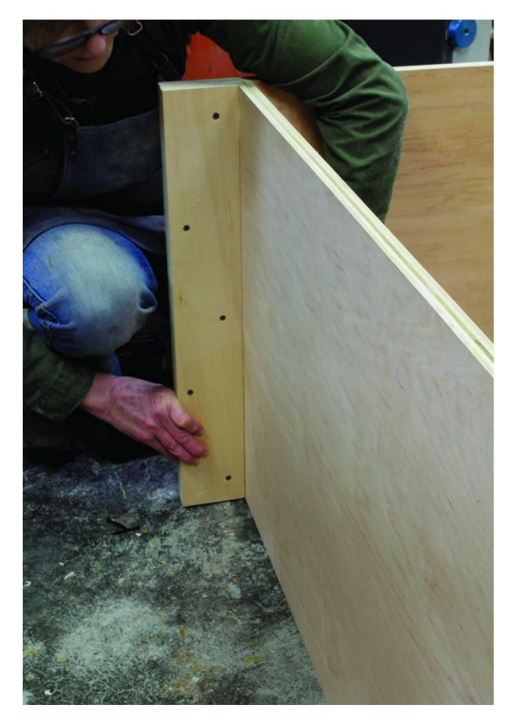
Maximize the efficacy of glue. Make sure the bottom face of the cabinet floor is tight against the top edge of the spacers; the bead of glue along the spacers' top edge will contribute to the cabinet's strength, especially if you are using plywood that's pre-finished only on the interior face and so offers few opportunities for gluing.
