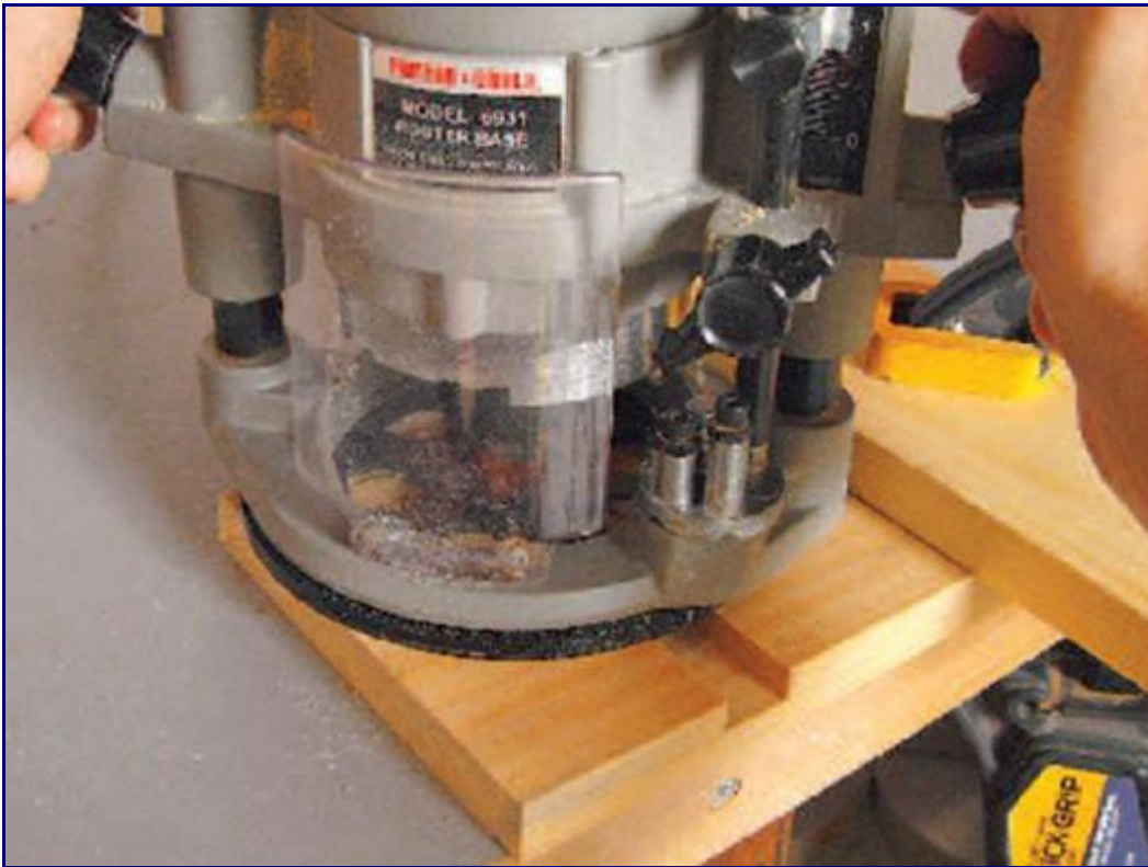
Routing the dado using a guide and plunge router
