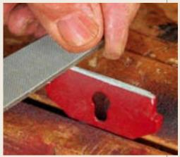
**Smooth the chipbreaker.** Rough casting and paint prevent many chipbreakers from making good contact with the blade. File down to flat metal (left). Bevel the leading edge (right) to create a tight joint with the blade, which keeps shavings from getting caught under the chipbreaker.
