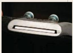
Close the throat. Make a dense hardwood shim (left) that fits between the frog and blade. The shim shouldn't be so thick that the blade no longer engages the adjustment screws. The tighter throat (right) makes for much smoother
