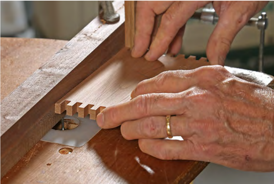
Groove for the bottom. To prepare for a bottom panel, Stowe routs \frac{1}{8} in. above the lower edge. Two parts get a stopped groove, two get a through-groove.
