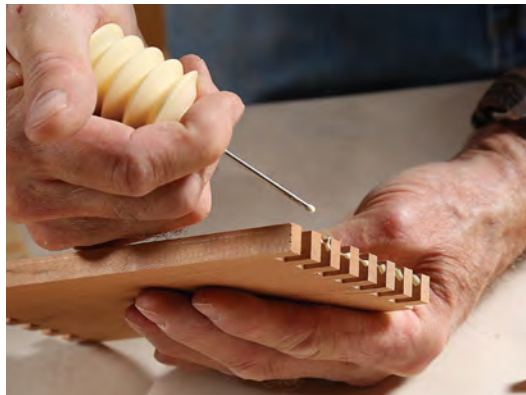
Glue the fingers. Apply a drop of glue to the edges where the parts slide together. The glue will spread as the fingers interlock.
