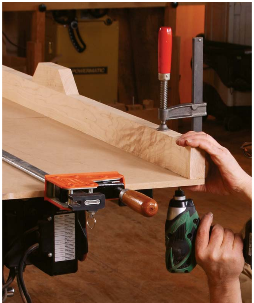
Screws hold the fence. With the front fence glued down, Turner drives a series of screws into pre-drilled holes to lock it in place. Its squareness is not critical.
