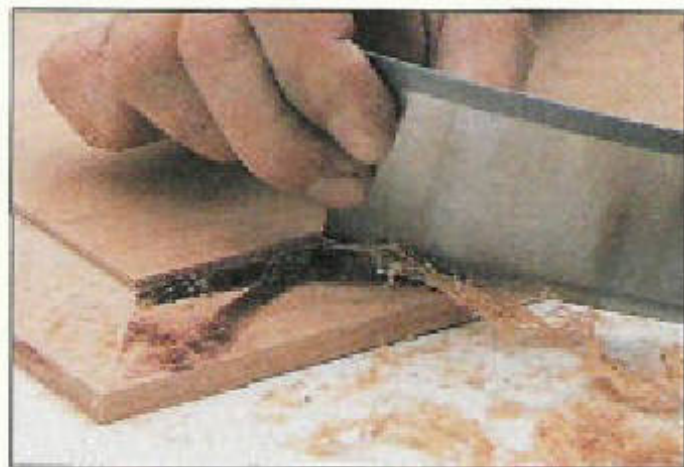
▲ Burn Marks. A hand scraper is the tool I reach for most often to remove stubborn burn and saw marks.
