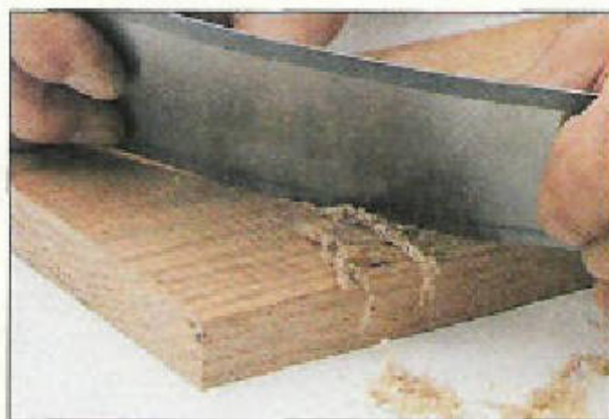
▲ Planer Marks. Hand scrapers can be used to quickly remove the ridges or marks left by a planer.
