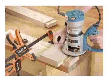
To steady the workpieces, stack and clamp parts for routing out the edge cheeks before clamping the assembly to the workbench.
