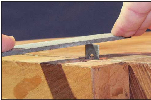
Filing the cutter to fit the string width
