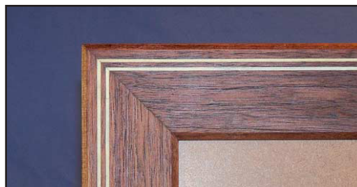
When both the string and substrate materials show, it's time to stop scraping
