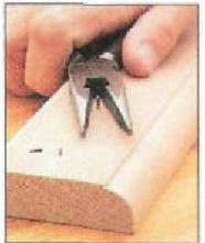
To keep layers aligned during glue up, nail a few wire brads in one of the layers. Then snip off the heads
