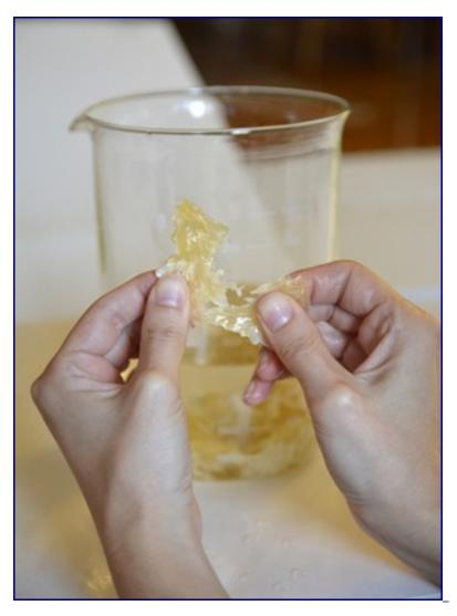
Once the bladders are sufficiently spongy, they should be kneaded into a homogeneous blob. The texture was kind of doughy at this point, and obtaining the blob was easier than I thought. Any hard bits should be worked into the dough. If there are a few remaining, they
