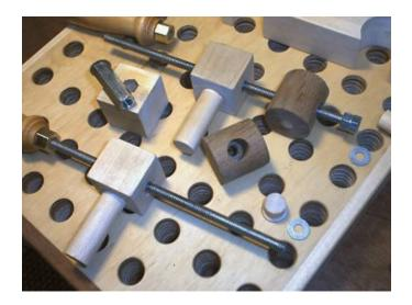
Sometimes, it is more convenient to clamp the work down onto the table, instead of sideways between jaws. My original plan was to embed a matrix of threaded inserts into the top of the table so I could use my holddowns. Then I had an inspiration. One threaded insert could be embedded in the end of a dowel and the dowel inserted from the bottom of the table, if it had a head so it wouldn't pull through. I already had one that I could adapt.
