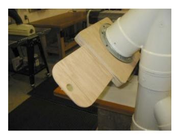
This is a close up of the flanges. This one is mounted to my miter saw hood, but it is the same thing I used on the gates.
