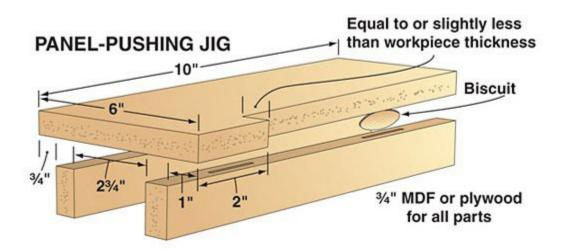
The jig raises the pressure point on the panel, holding it tightly against the fence, and protects my fingers from the blade. I used biscuits to join the runners to the jig, but you also could dado the jig and glue the runners into place. (Note that the runners should be taller than the blade height.)
