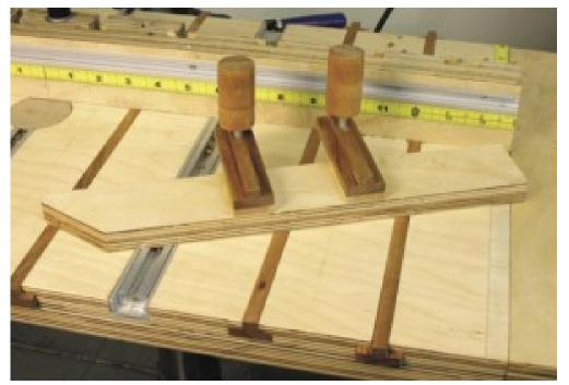
For working with taller objects, a taller fence (part K) is handy. By utilizing the T-
