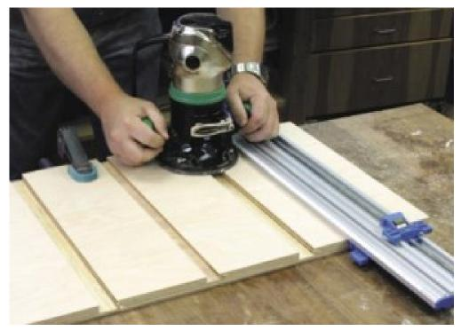
After making my centered  $3/4'' \times 3/8''$ -deep dado, I cut both the side  $1'' \times 1/2''$ -deep dados using two passes with the same bit.
