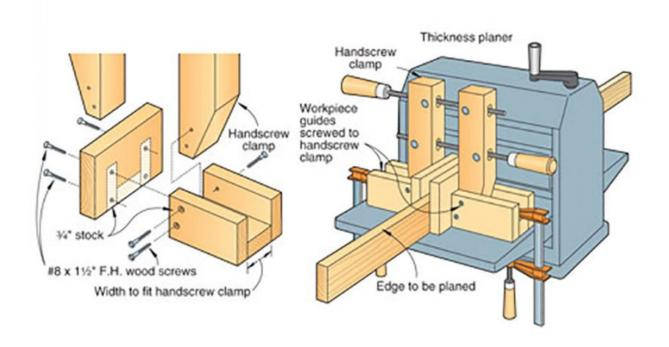
With an old handscrew clamp and some scraps of hardwood, you can set up your thickness planer to mill uniform-width door or cabinet stiles, rails, and other pieces with jointer-smooth, square edges.
