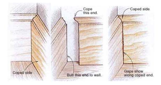
If a coped joint opens up, the crack will be obvious when viewed parallel to the uncoped piece and nearly invisible viewed parallel to the coped piece.
