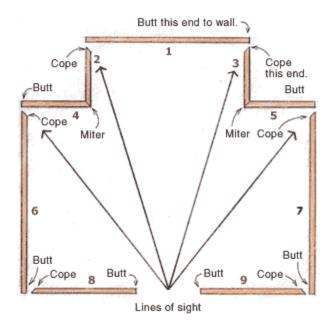
As with trimming doors and windows, sequence of installation is also important when running trim around a room, whether it's baseboard, chair rail or crown molding. For instance, I'm right-handed and can generally do a faster, neater job of coping the right end of a board than the left end (coping is an alternative to mitering joints at inside corners). Consequently, I often prefer to work from right to left around a room.
