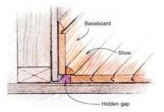
Moldings hide the gap: Floorboards don't have to be a uniform distance from the wall. As long as the base/shoe molding covers it, the gap can vary.
