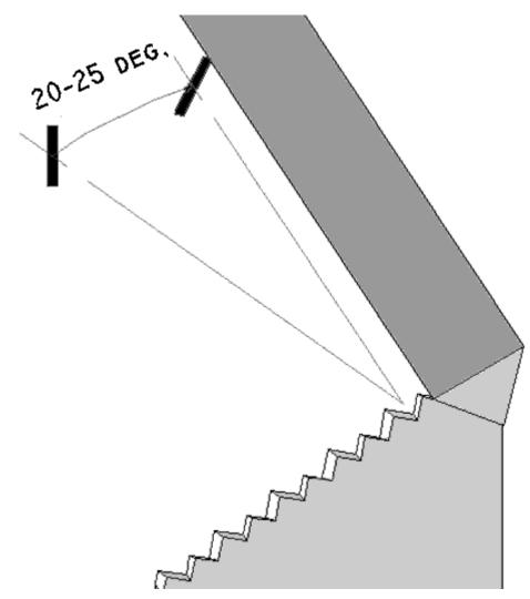
This diagram shows a fleam angle of 20 to 25 degress. Every other tooth gets filed to the prescribed angle, then the saw is flipped and the remaining teeth are filed to a mirrored angle. It's this angle that forms the slicing points shown in the diagram above - you can sort of make it out in the teeth shown in this diagram. There will be more on this angle in the next page, where you will also see this same diagram again.
