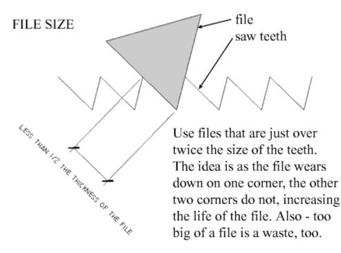
I find I can use a file for shaping teeth for quite a while, but for final sharpening it really pays to use a nice sharp one. For teeth finer than 16 PPI, you can also look into using a needle file. I've not done this, but others have reported success to me using them. Files less than 6" long can be difficult to find in your local hardware store - I've had good luck getting them from Lee Valley and McMaster-Carr.
