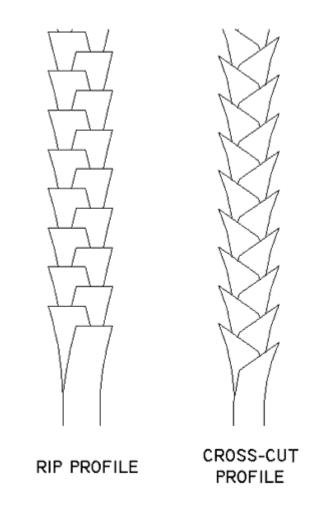
Dad always told me that you could slide a needle down the valley that forms between the teeth of a well-sharpened crosscut saw. I say this just to point out the slicing cut that it makes. Personally, I have used each for cutting dovetails - and I can't say I prefer either way. Regardless, a cross-cut saw is needed for making some shoulder cuts for tenons, so having one of each seems like a good idea.
