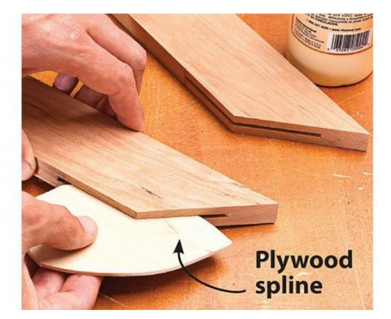
Cut each slot with the short edge of the miter cut against the saw table.
