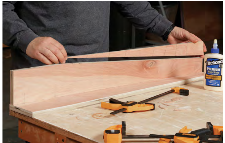
Use tapered offcut as a caul during glue-up. Clamping tapered parts, like these legs, can be tricky. Use a tapered offcut to direct clamping pressure square across the joint.
