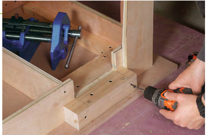
Vise needs blocking. These blocks give you a place to drive the bolts for attaching the vise. They also bolster the front apron, which will be under a lot of stress from the vise.
