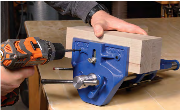
Hardwood jaw pads protect work. Rip these wide enough so they extend just above the top of the bench. McBrien uses maple here, but any hardwood will do.
