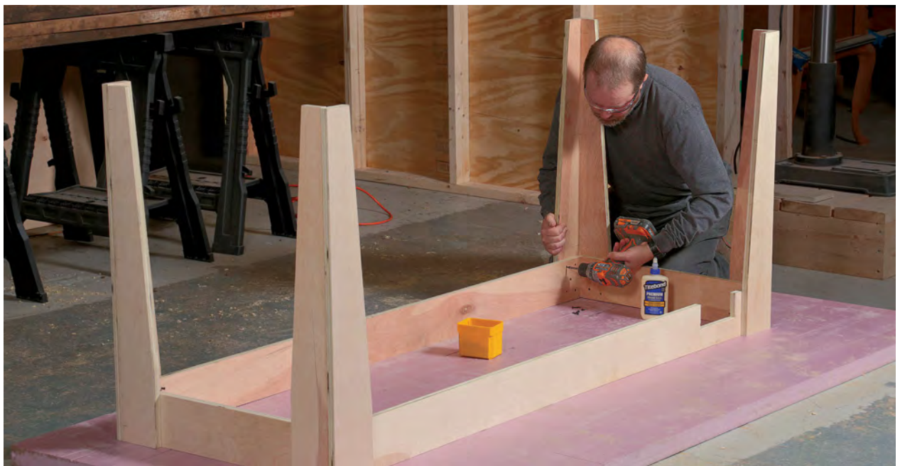
Use tapered offcut as a caul during glue-up. Clamping tapered parts, like these legs, can be tricky. Use a tapered offcut to direct clamping pressure square across the joint.
