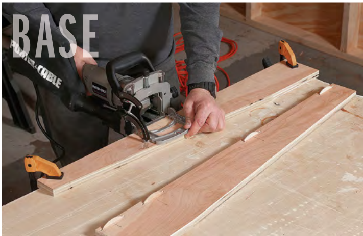
Biscuit the leg assemblies. After tapering, the two sides of the leg assemblies are glued together. Biscuits help with alignment and strength.
