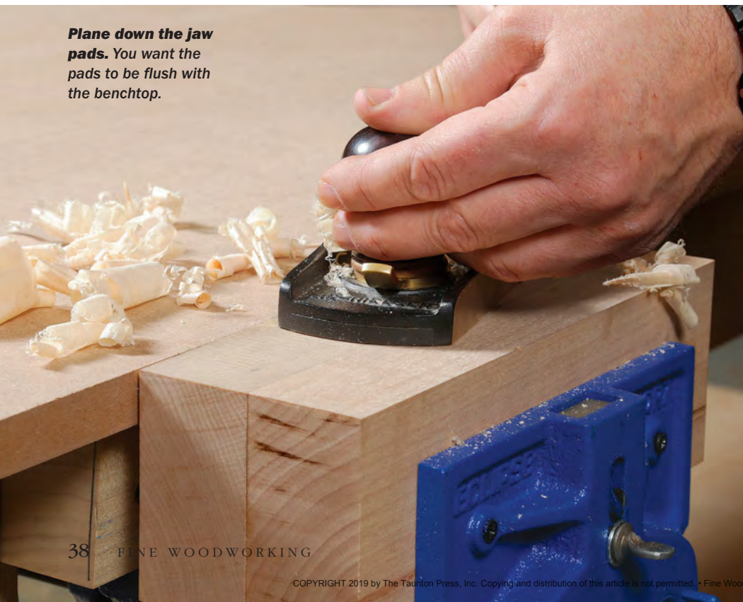
Hardwood jaw pads protect work. Rip these wide enough so they extend just above the top of the bench. McBrien uses maple here, but any hardwood will do.
