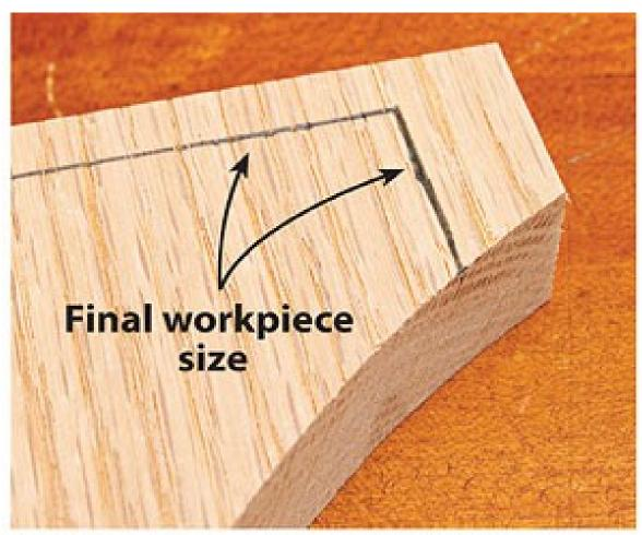
By leaving extra material to back up the bracket point, any tear-out will happen on the waste side of the line.
