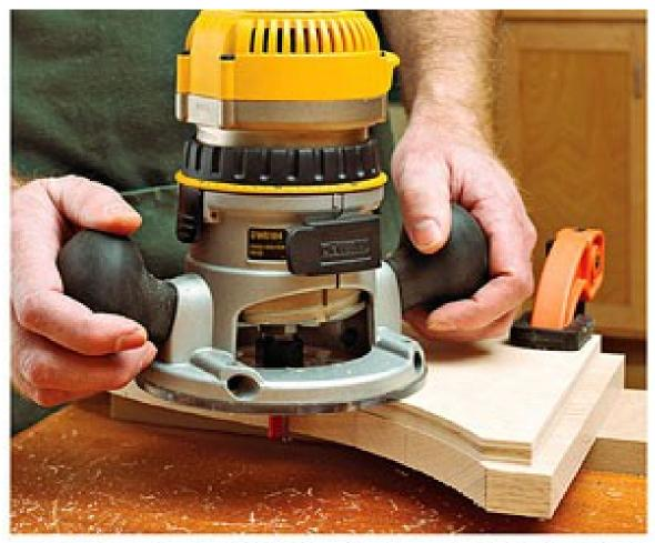
Leave about 1/16" of waste material so the router needs only to shear off fine shavings rather than large chips that cause tear-out.
