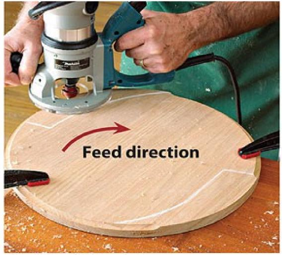
Climb-cut the danger zones, holding the router firmly to guard against jerking.
