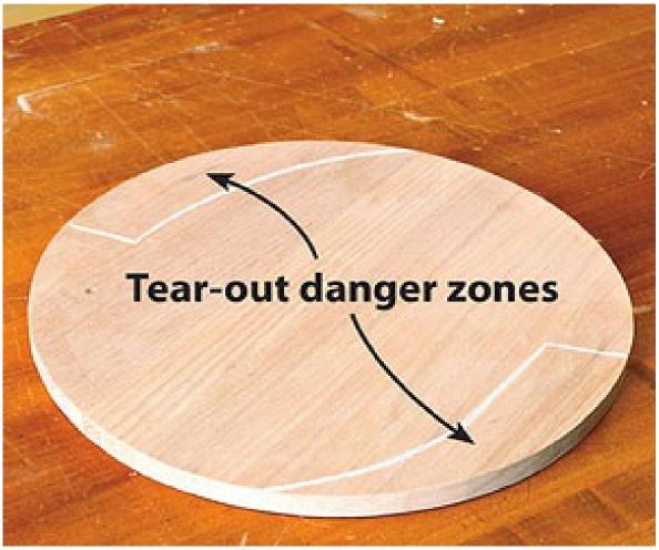
Danger zones feature grain that parallels the edge and is prone to tear-out.
