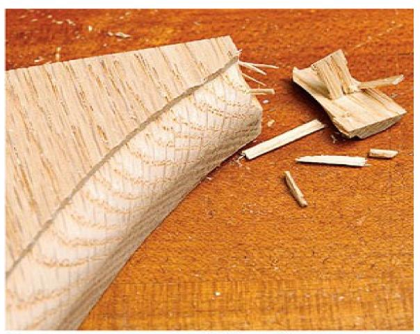
The unsupported tip of this shelf bracket broke away as the router made a simple round-over beaded profile.
