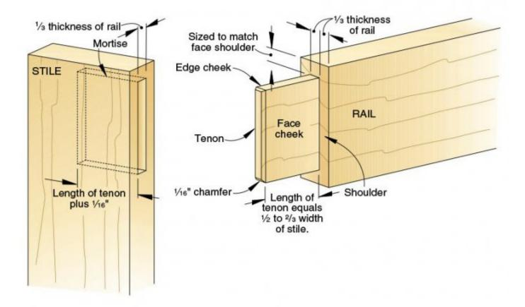
Specific mortise-and-tenon size will vary by application. As a general guideline, make the tenon about 1/3 the total thickness of the tenoned workpiece, and about 1/2 - 2/3 as long as the width of the mortised workpiece. Though it's not structurally necessary, cutting a shoulder adjacent to the rail's edge as well as the face allows you to completely hide the mortise. To save setup time, size the edge shoulder the same as the face shoulder.
