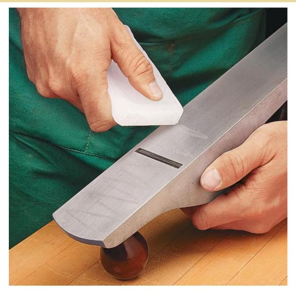
Other than keeping blades sharp, applying some wax may be the easiest thing to help cutting tools work better. Many old-time woodworkers kept a chunk of wax nearby as they used their hand planes and saws. A few "scribbles" of wax on the bottom of a hand plane makes it slide easily across a workpiece.
