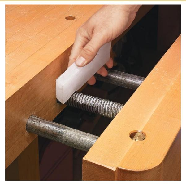
Paraffin (canning) wax is a solid bar that's slippery and forms a medium hard film. You'll find it at most grocery stores. Besides making screws easier to drive, I use a bit of wax on adjustment rods like the threads on a workbench vise. Then run the vise in and out a couple times to work the wax in and you'll quickly notice a difference.
