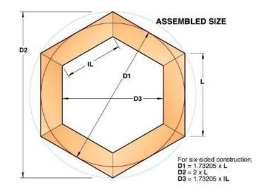
And if you need to know the diameter of the opening in a ring, shown as D3, just multiply the length of the short edge of the segment (IL) by the appropriate inside-diameter factor.
