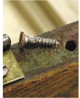
Seasonal wood movement can eventually crumble the fragile interface between the wood and the threads of the screw, enlarging the hole.
