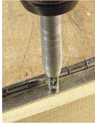
The Vix bit has a self-centering spring loaded guide that makes it invaluable when drilling holes for hardware.
