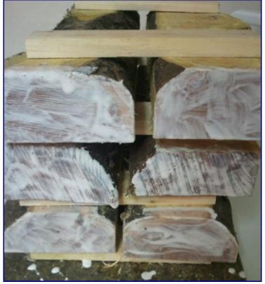
This small stack of Buckthorn (Rhamnus cathartica) half-logs has just been cut, stacked, stickered, and sealed with a water-based wax emulsion coating.
