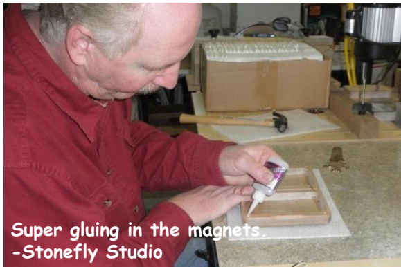
Inserting magnets into recessed holes. -Stonefly Studio
