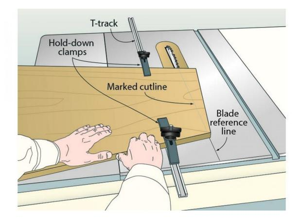
fAter reading Alan Schaffter's tip ("Arrow-straight cuts for oddshaped parts," *WOOD* magazine issue 193, Oct. 2009), I thought I'd send in my own down-and-dirty "sled" for cutting irregular panels. Mine consists simply of two hold-down clamps attached to T-track with T-bolts and star knobs (Rockler item 25736, 800-279-4441, rockler.com).
