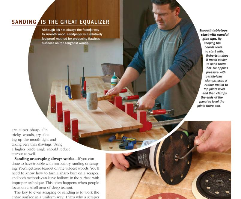
**Try a firmer pad.** Firm sanding pads are available for many sanders. They stay flatter in use, a big plus on large surfaces and those with figure or defects.
