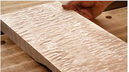
**Use sharp blades and skew the board.** Roberts installed sharp knives on his jointer, skewed the slab of quilted maple as far as possible to create a shearing cut (top), and got amazing results this time.
