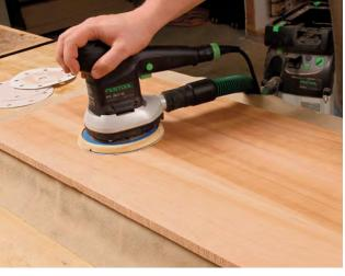
Sand in a uniform pattern. To avoid creating hollows and leaving behind scratches from previous grits. work the panel in a uniform pattern with each new disk. Be sure to attach a vacuum to the sander, keep it level, and don't add any pressure beyond the weight of your hand and the sander itself.
