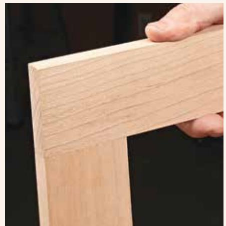
▲ Another test for a tenon is to dry fit the joint and raise the mortised piece. The workpiece should stay in place.
