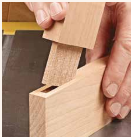
▲ A properly sized tenon should fit into the mating mortise with moderate hand pressure or light mallet taps.
