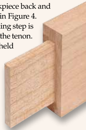
▲ Here's the result of cutting a tenon with a dado blade.
