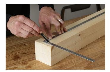
Connect the centerlines. Set a long straightedge on the marks on both ends and trace. Do this on all four faces.
