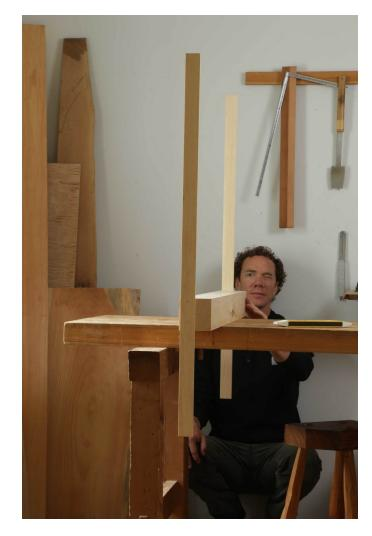
Check your lines with winding sticks. Align two long wooden straightedges with your layout lines and tack them in place. Use them to verify your lines are coplanar.
