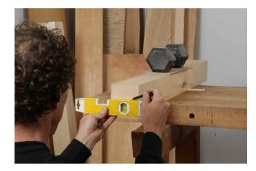
Mark level and plumb across the middle of the ends. Hunter keeps a weight on his workpiece to keep it from slipping during layout.
