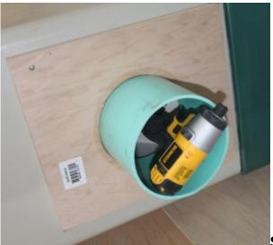
**Simple to make**. Take a 6" piece of PVC, set it on a piece of plywood or MDF, trace a line around the outside of the pipe, and cut the hole. Set the PVC in the hole and caulk it on the outside. Then place " foam weather stripping around the perimeter of the plywood, and use sheet metal screws to attach to your tool. If the stock port opening on the tool isn't large enough, or isn't there, use a jigsaw with appropriate metal cutting blade to modify or create the opening.
