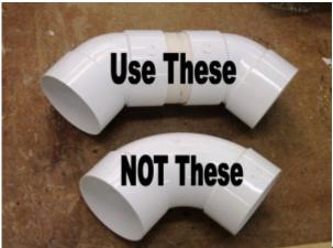
**45s not 90s**. Rather than a short radius 90 degree turn, incorporate two 45 degree bends with a section of straight pipe in the middle, which will allow the particles to scream right through the turn. If you can find elbows that are specially designed as "long sweep" elbows, you can use these, but they are not commonly available in my area.
