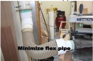
**Minimize the flex pipe**. Run hard pipe as close to the tool as possible, and use just the flex pipe you need for convenience in case you need to move the tool. Also, choose a good quality flex pipe with smooth interior walls that was designed specifically for dust collection. Some of the cheaper stuff I have used is extremely rigid, making it terrible to work with. Good flex pipe is expensive, so I am sufficiently motivated to minimize it for that reason as well.
