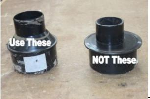
**Tapered vs. abrupt reducers**. When you need to drop down to a smaller duct size in line, use a reducer with a smooth taper rather than an abrupt reduction. This will promote better air flow and reduce turbulence in the pipe.
