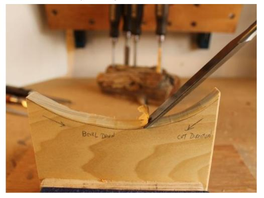
After laying out the curve on the workpiece, clamp it in the vise and remove the bulk of the waste with a coping saw. Cut with the grain, using short mallet strokes as you get closer to the line, advancing the cutting edge 1/4" or so each stroke. As you chop, raise or lower your arm to keep the cutting edge from going beyond the layout line. The final smoothing can be
