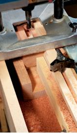
Rout mortises making stepped cuts for safety. Each pass should be  $\frac{1}{4}$ " to  $\frac{3}{8}$ " deep. Pull the router toward you so the bit rotation forces the router's edge guide to the side of the jig.
