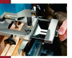
Set-up can be a snap. With the bit set to just clear the work piece, set the stops for the router, then adjust the router's edge guide to the mortise layout lines.
