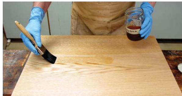
5 More coats. Brush a wet coat of wiping varnish onto the surface. You don't have to be too careful how you brush because the dry brushing will smooth things out.
