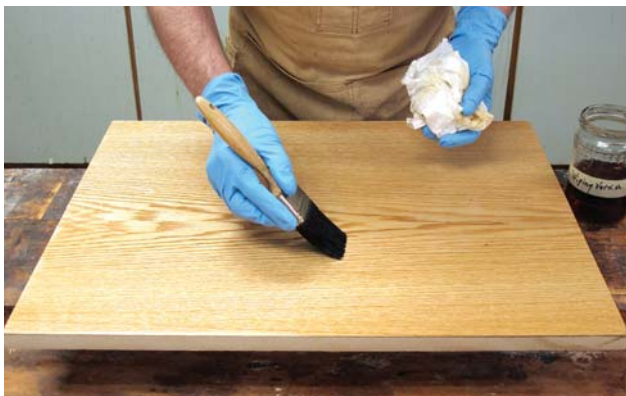
3 Reflected light. Watch what's happening in a reflected light. Your goal is to get an even thickness of finish without puddles on horizontal surfaces or runs on vertical surfaces.
