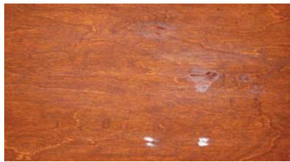
Finish residue. When stripping a finish, don't be fooled by stain that isn't removed. It's rare that all the stain comes out of the wood. Instead, look for remaining shiny areas that indicate you haven't removed all the finish.
