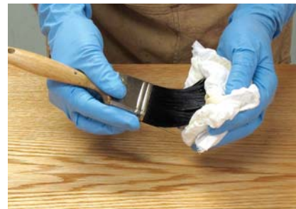
1 'Dry brush excess' method. With the surface wet with wiping varnish, dry your brush on a clean cloth.
