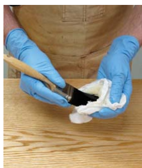
7 Dry the brush. After each pass, dry your brush on a clean cloth. If you decide to dry-brush the surface a second time, you can make more than one pass before drying the brush. You'll get the feel very quickly.
