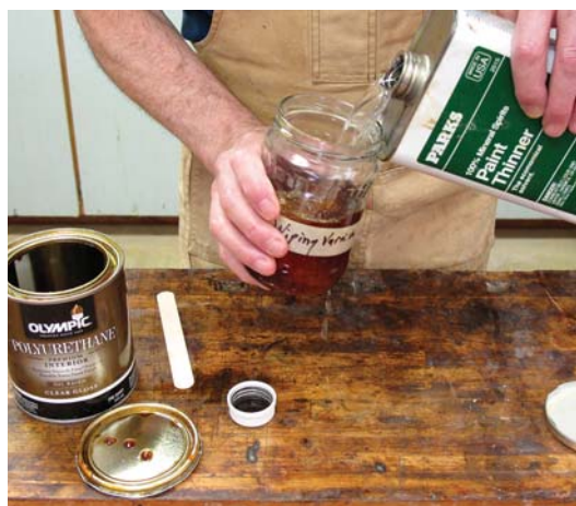
Make your own. To make your own wiping varnish for this exercise/project, pour approximately equal amounts of oil-based, gloss polyurethane and mineral spirits into a clean wide-mouth container.
