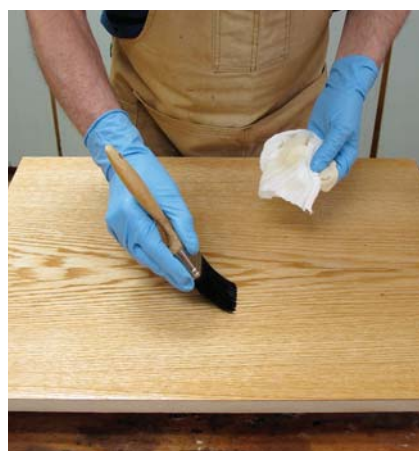
6 Dry brush excess. With the entire surface wet, begin lifting some of the wiping varnish by brushing over with a dry brush.
