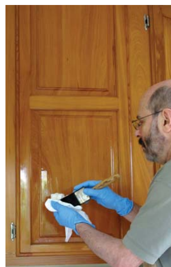
5 More coats. Brush a wet coat of wiping varnish onto the surface. You don't have to be too careful how you brush because the dry brushing will smooth things out.
