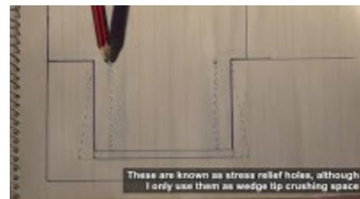
A small hole is bored at the base of each saw kerf, which provides stress relief and space for the wedge tip to crush if necessary
