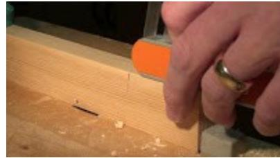
Check the angle with the toe of the bevel gauge
