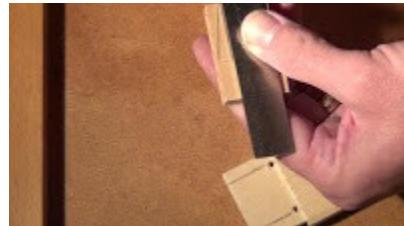
The second wedge can utilise the sloped cut off the first
