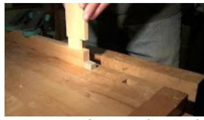
Gradually push the tenon into the mortise, forcing the wedges further into the saw kerfs
