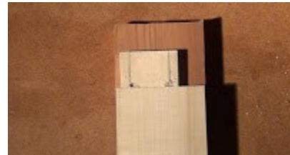
Drill the two holes, right up close to the tenon shoulders
