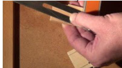
With a bevel gauge set to the back cut angle (1:7 is a reasonable guide), mark out the first wedge. Remember to add the width of the saw kerf to the wedge
