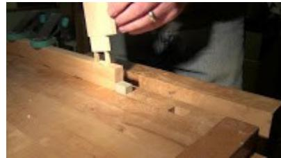
Insert the tenon, with wedges pinched in the saw kerfs, into the mortise
