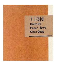
Trade names: None Garnet is an excellent choice for final sanding end grain and blotch-prone wood. Garnet's peculiar tendency to burnish wood--close off pores--makes a stain penetrate far more evenly though less deeply.
