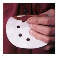
**Discs don't flex, they break**. The adhesive and backing on a random-orbit sanding pad can crack if the disc is folded like ordinary sandpaper.
