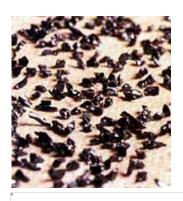
**Abrasive grains are little sawteeth**. This is 24-grit silicon carbide sandpaper before a size coat has been applied. It is easy to see how sharp the particles are.
