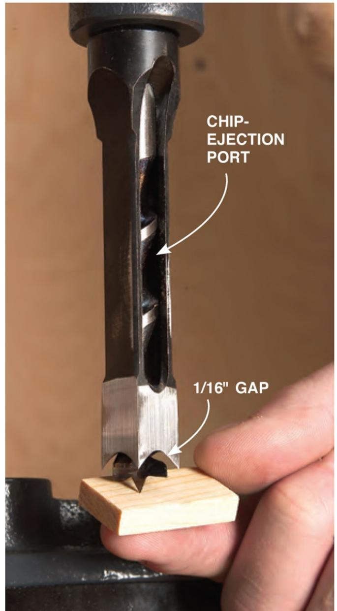
**4. Leave a gap.** Position the auger bit with its cutting head about 1/16" away from the domed inside surface of the hollow chisel. Don't jam these two parts together. The gap is essential, because it allows shavings cut by the auger to be lifted into the hollow chisel and ejected. If the gap is too small or too large, the trapped shavings will bind the bit. Then reposition the chisel.
