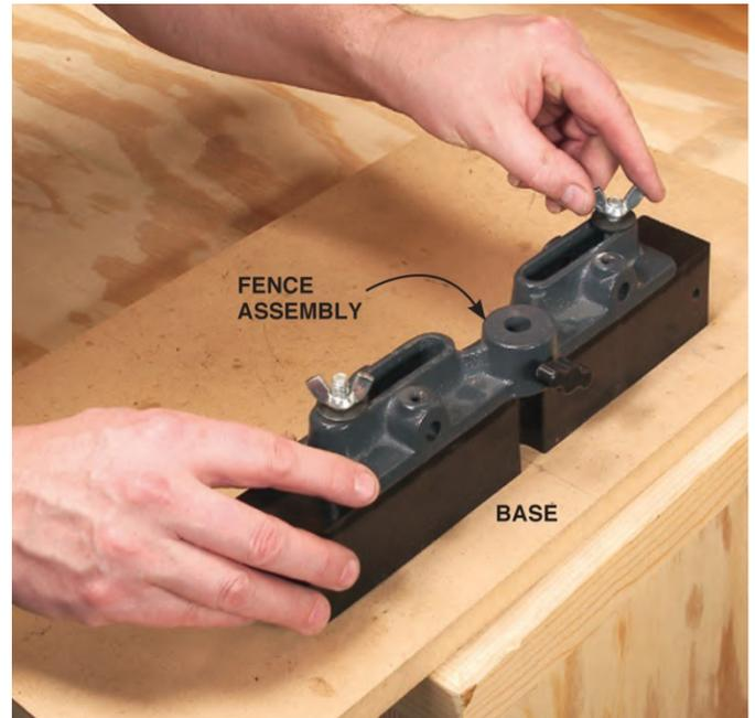
**2. Mount the mortising fence on a separate base**, rather than fastening it directly to the drill press table. Then clamp the base to the drill press table. This setup makes the fence easy to adjust; so positioning the workpiece is a breeze.
