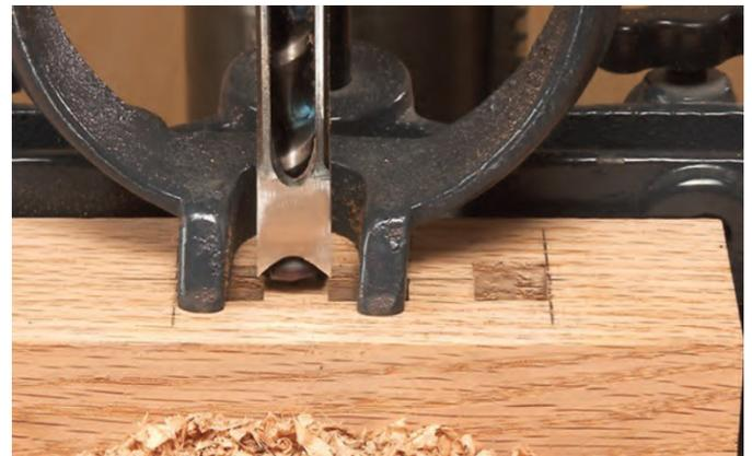
**12. Establish the ends** of the mortise first. Then clear out the middle. Always engage all four sides of the chisel or two opposite sides. Apply steady pressure and advance the cut slowly. Don't push too hard. Match your feed rate to the cutting action of the auger by watching the flow of chips exiting the chisel. Easy—but firmly—does it.
