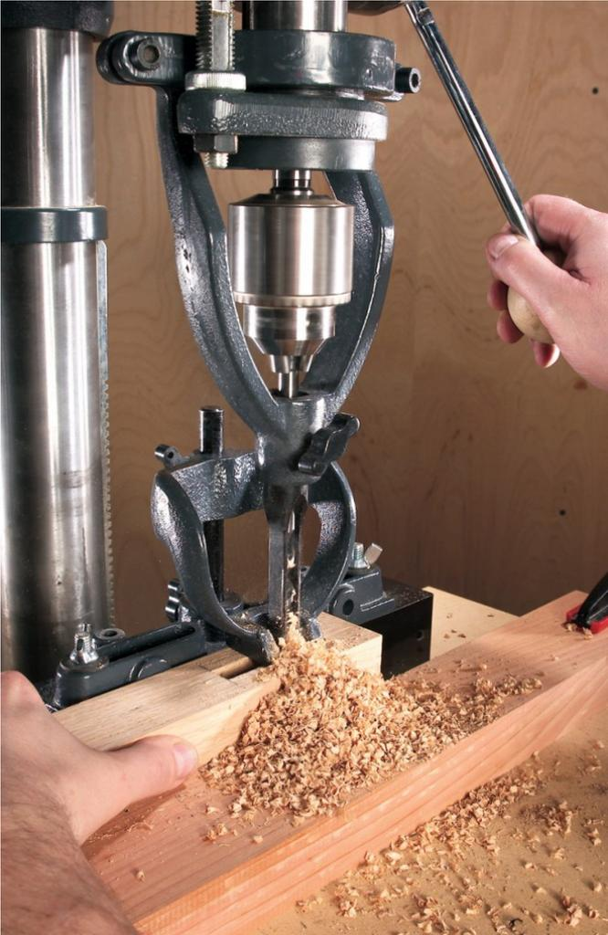
Even though they're sexy, benchtop mortising machines aren't the only power-tool option when it comes to cutting square-shouldered mortises. A drill-press mortising attachment can be just as effective and it costs a lot less. I'll show you how to tune any out-of-the-box mortising attachment so it's easy to install and a joy to use. Mortising attachments are available for almost every drill press.
