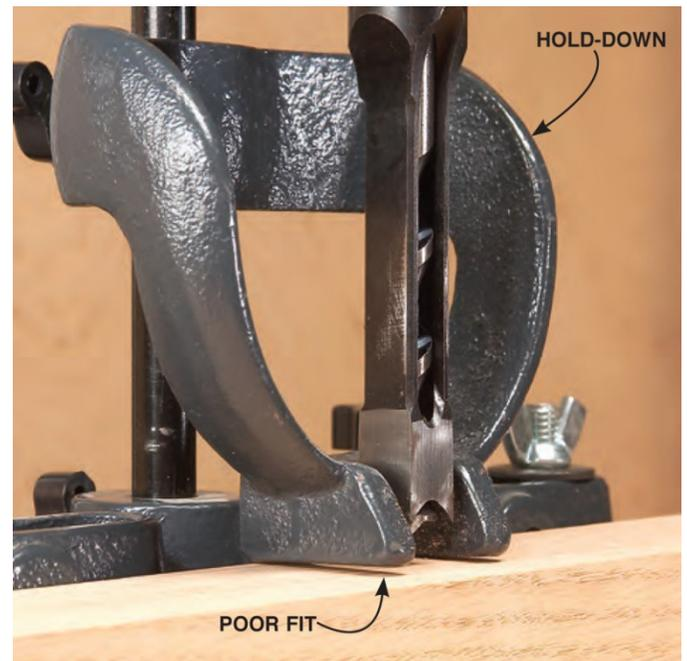
**6. Check your hold-down.** If it doesn't sit flat on the workpiece, grind or file it until it does. A poorly fitting hold-down won't hold the workpiece firmly enough against the base. While you're mortising, any workpiece movement can bind the bit in the mortise and wreck your setup—or the bit.
