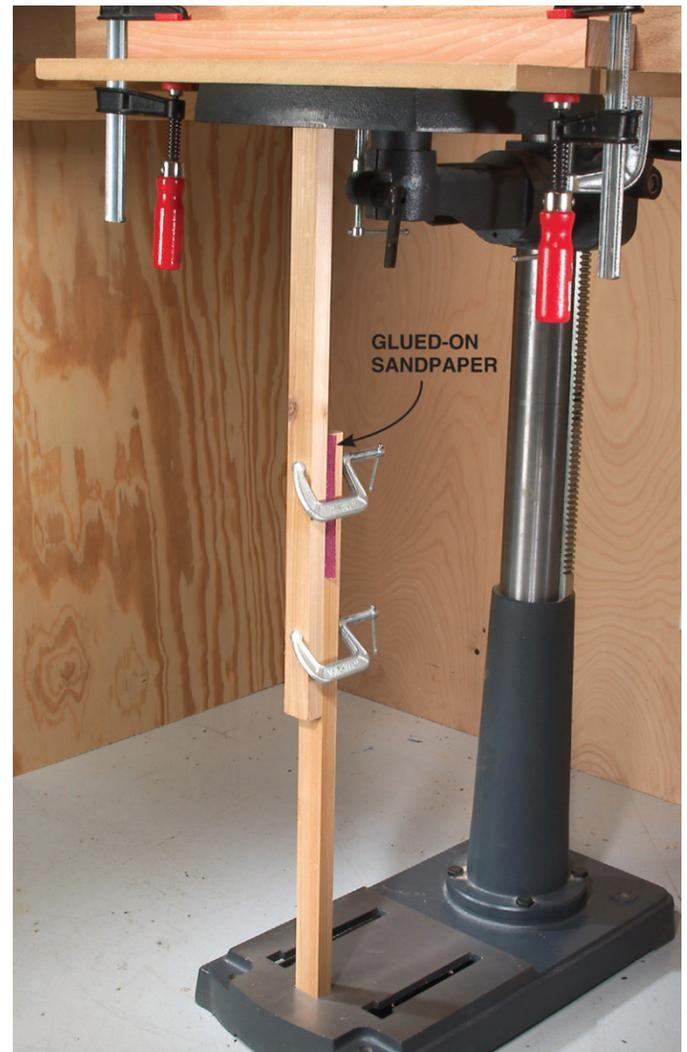
**8. Stiffen the table** with a brace. On many drill presses, mortising exerts enough downward pressure to flex the table. Like workpiece movement, any table movement will cause trouble. If the table flexes, the chisel will bind in the mortise. A two-part adjustable brace is much easier to install.
