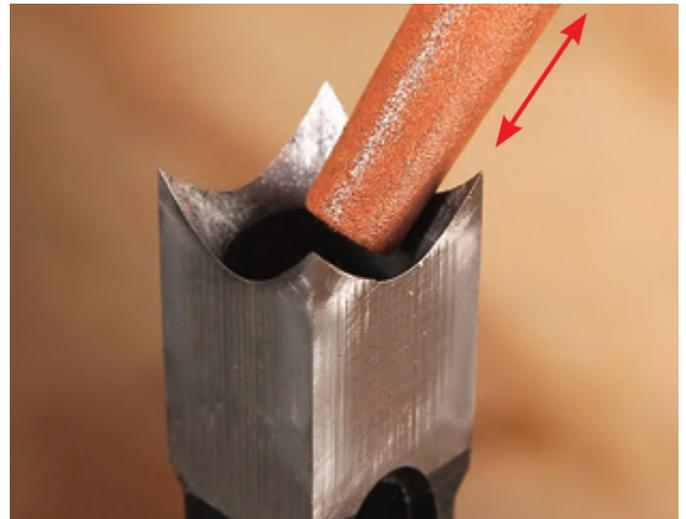
**Sharpen the hollow chisel's inside bevels** using a round slipstone or rotary tool. Grind from corner to corner while holding the stone flush against the bevel.
