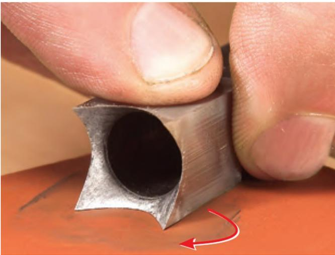
**Hone the outside faces** lightly on a flat stone, using even pressure and a circular motion.
