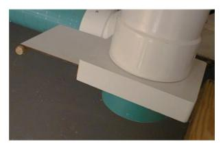
This particular blast gate (shown installed) was attached to a wye fitting that is basically pointing down at 45 degrees. The gate is a piece of 1/4" paneling that is at least 1/16" undersize on thickness and a handle has also been attached to it.
