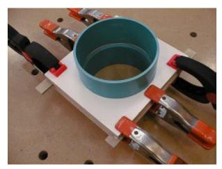
It is also important in a design such as this that the gate does not fit too snugly (thickness wise) between the halves. A snug fit may actually prevent a closed gate from being sucked up to the vacuum side to provide a good seal. I have found that a gap of 1/16" or more creates a very good gap.
