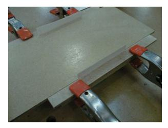
The easiest way to create a space for the gate itself is to just space the halves apart by the proper amount. In this case I am using the thickness of the guides (1/4") to control this. Because of this, my gate material needs to be a little less than 1/4" thick to slide in and out well, more on that later.
