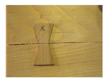
Using a small brush, apply a thin layer of glue to all of the surfaces of the mortise and to the bottom of the spline. I usually don't glue the sides of the spline because it all gets peeled off when it's being driven in. And less glue to clean up is less glue to clean up ('nuff said). Put the spline in the mortise and using a scrap to protect the surfaces, tap it in with a hammer. Listen as you tap it, the sounds it makes will tell you how deep you are and when you've reached the bottom.
