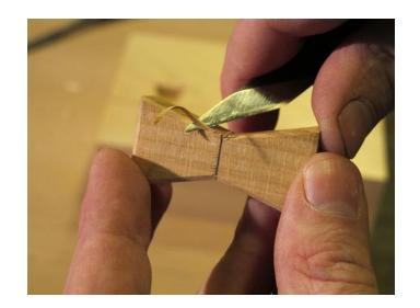
If the fit is good, carefully pull it out. Using a knife or chisel, chamfer (bevel) the inside edges of the spline. This will help it slide in straighter, keep from damaging the edges of the mortise and leave a little clearance in the corners for glue squeeze-out.
