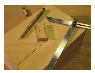
Start with making the spline. I'm using a piece of cherry measuring 1" wide 2" long and 3/8" thick (it's important that the grain runs the length of the long dimension). Using an adjustable square, I mark the center of its length, and then 1/4" in from each side. Then, using an angle gauge (I knew I forgot something in the layout tools article), draw lines from the outer corners to the center marks.
