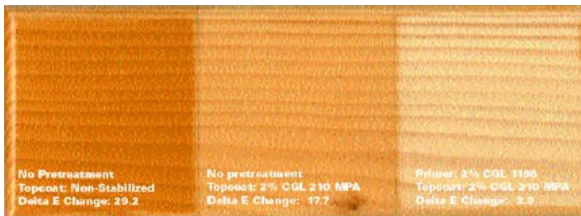
Figure 7: Panel Appearance after 1,500 Hours UV A-340 Exposure Topcoat: Clear Alkyd Varnish, Primer: Aqueous Solution
