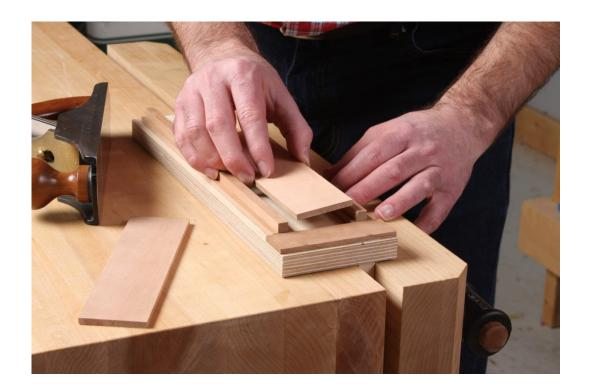
**Drop in the stock.** It's best to start with boards that are just barely thicker than 3/16". I make them at the bandsaw, cutting them around 7/32" thick. One face should already be jointed and planed clean because, if you plane it after using the jig, the board is no longer the desired thickness.
