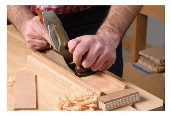
**Plane away.** The guides not only keep the plane moving straight ahead, but alos prevent it from swerving off course and cutting into the rails. Just keep planing until you no longer get any shavings. The board is now a consistent thickness.
