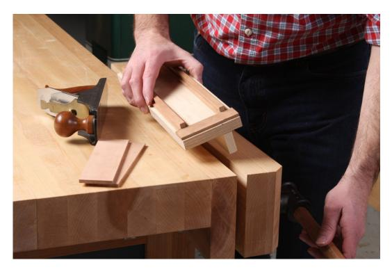
**Small Planer.** The rails of this jig are spaced just wider than the blade of a No. 4 smoother. They're just a hair thicker than 3/16", so that boards planed with the jig end up 3/16" thick. A cleat on the bottom is clamped in a vise to hold the jig still during use.
