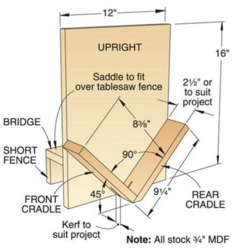
Build the jig from 3/4 " BB and not MDF as in the picture. Bevel one end of the rear cradle at 45-degrees, then glue it to the upright at a 45-degrees angle to the bottom edge of the upright. As you glue the front cradle in place, check that the two cradle pieces are 90-degrees to each other.
