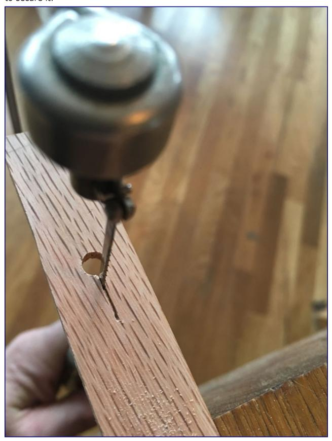
At the other end of the bow, make a keyhole-like notch to grasp and hold the string. First drill the same-diameter hole as earlier. Then saw a slot about 3/4" long that extends down the
