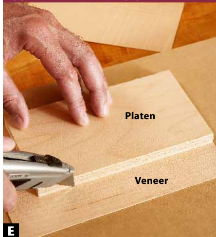
E Hold a plywood platen in place on each piece of veneer and, using a fresh blade, cut around the platen.
