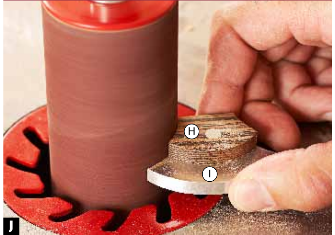
J Sand the sides of the handle assembly (H/I) on progressively finer sanding drums to achieve the sheen you desire on the metal.
