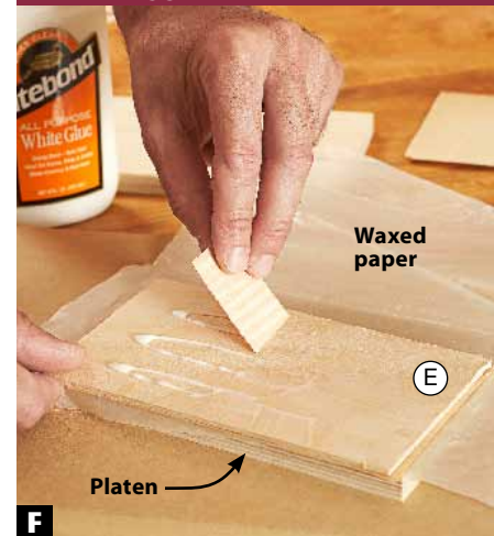
F White glue allows for a longer working time. Spread an even coat, then position the veneer flush with the platen edges.
