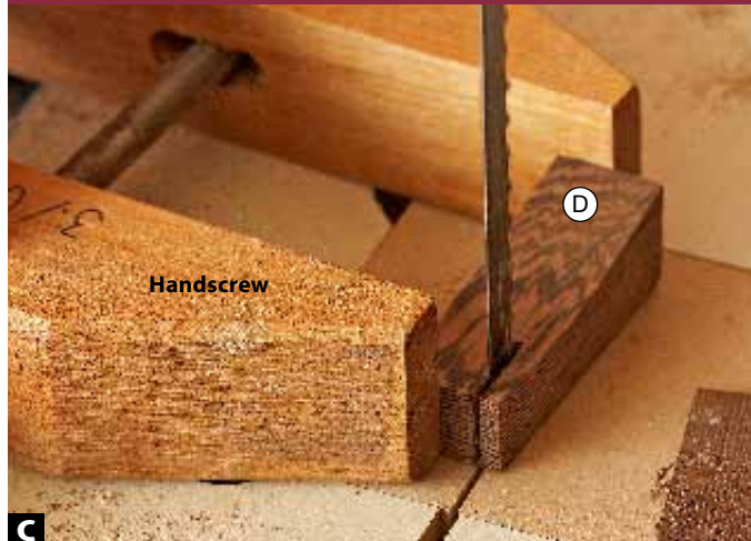
C Safely grip each foot (D) in a handscrew. Bandsaw just outside the line; then lay out the curve on the adjacent face.
