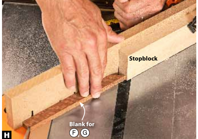
H Position the miter-gauge head as shown so the workpiece presses against the stopblock throughout the cut.
