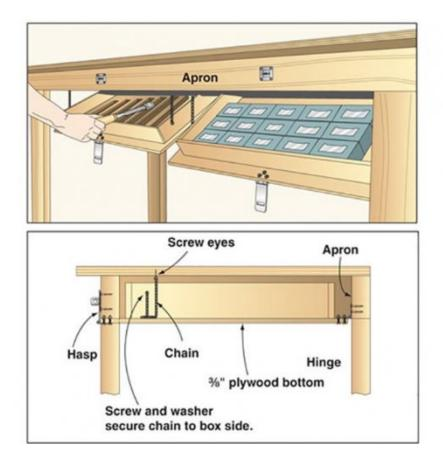
I discovered a simple way to make use of the space underneath my workbench top and behind the skirt without re-engineering the base for drawer boxes. To use the space, I built drop-down storage compartments, as shown at right, to hold small tools and to organize my fasteners.
