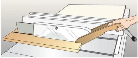
I feel safer performing tablesaw rip cuts with this double pushstick that I came up with—two pushsticks connected with a 1  $\frac{1}{4}$ " dowel that's longer than the width of the blade guard. It allows me to cut narrower pieces without getting my fingers close to either side of the spinning blade. Plus, it straddles my blade guard, giving me one more incentive to leave the guard on the saw.
