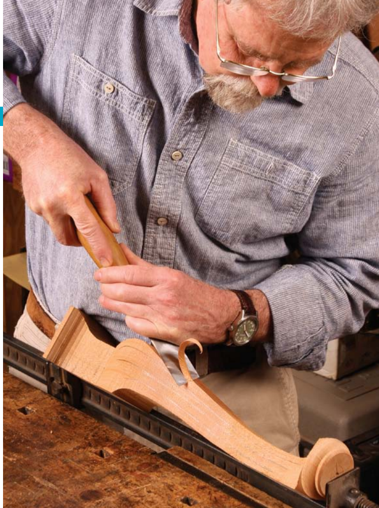
Go bevel down on concave surfaces. Like the short sole of a spokeshave, the bevel has no trouble following the curve.
