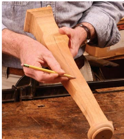
Start with layout lines. Lowe draws a center-line and two quarter lines on all four faces, so he'll know how much to material to remove.
