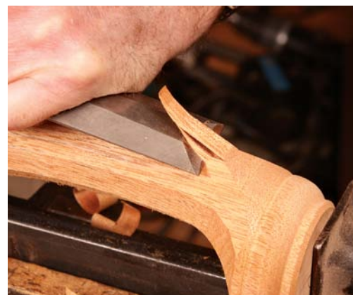
Stay in control with short cuts. They prevent the chisel from cutting too deeply and causing tearout.
