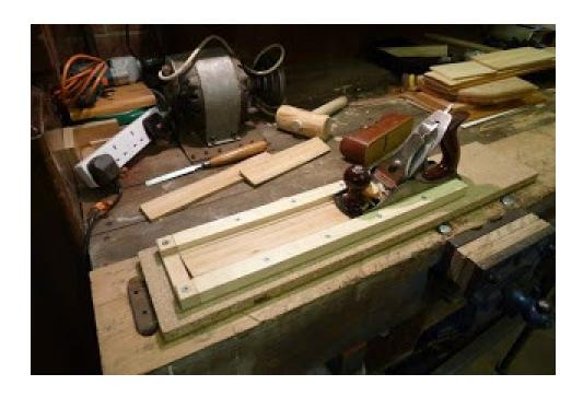
Here is a simple a jig for hand planing to exact thickness, in this case box sides. This is a design which has the plane riding on two narrow edges which are just outside the cutting area of the blade, so restricting the depth of cut and giving a consistent even thickness. The depth can be shimmed to suit different thicknesses and you can build the jig to any length. The only restriction is the width of your plane blade.
