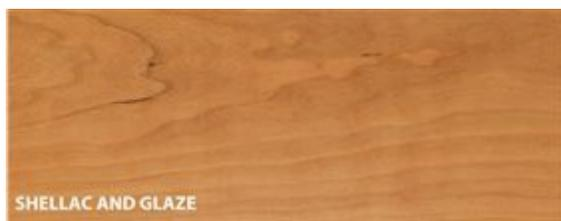
**Shellac and glaze adds rich color and minimizes blotching.** Shellac seals the wood so the glaze, which is thinned oil paint, adds color evenly. You can wipe the glaze hard, or feather it, leaving more in some spots than others. Glaze is great for disguising light sapwood.
