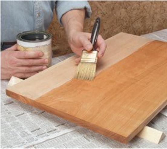
**1. Seal the surface** with dewaxed shellac. On cherry, a single thin coat (2 lb. cut) allows some glaze to lodge in the pores. This looks odd to me, because cherry's pores aren't naturally dark. Two thin coats, sanded between, keeps color out of the pores.
